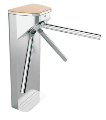
IDT-B2000 (semi-automatic tripod turnstile) is driven by DC brushless motor, one can easily pass with very less passing resistance. It has several working modes such as bi-direction, and single direction and all the modes can be set by using the buttons on the main control board. Beams will fall automatically when power is off and auto rise when power is on or auto stop on obstacles. It can also be integrated with function and face detection biometrics for no-touch use.
